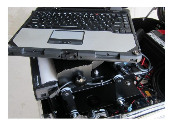
The FMS Accessories articulated mounting base is designed to attach directly to the threaded stand-off's inside a standard Harley-Davidson radio box. There are four pre-drilled holes in the base plate that should line-up with those four stand-off's inside the radio box. Use the same ½" x 20 TPI bolts that attached the cover plate inside the radio box.
