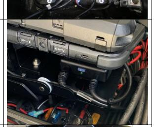
Attach the laptop using the two Velcro strips provided. Clean the base of the laptop where the Velcro will attach using the included alcohol pads. It is recommended to "test fit" the laptop only exposing a small amount of the Velcro adhesive and make sure you know it is in the right place. Secure the full adhesive length once you know it is where you want it to be.
