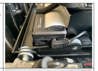
Attach the Brother PocketJet printer to the printer housing using the Velcro tabs provided. If battery access is needed, you may wish to carefully cut the Velcro strips as they cross over to the battery on the printer. The Velcro strips keep the printer not only in place while riding, but also from rocking or "torqueing" when it feeds paper, so the Velcro needs to span the full width of the printer.
